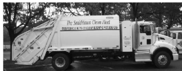
Figure 25. Smithtown 2010 Kenworth T440 CNG refuse truck with pedestal mount fuel system
