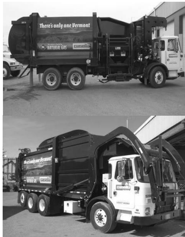
Figure 21. Autocar dedicated CNG refuse trucks with Cummins-Westport ISL G CNG engines in front and side-loader configurations.
