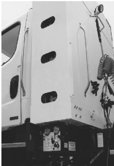
Figure 9. Compressed natural gas vehicle storage tank configurations: behind the cab, on the roof, or within the chassis
