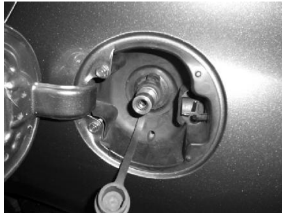
Figure 6. P36 CT1000 compressed natural gas receptacle
