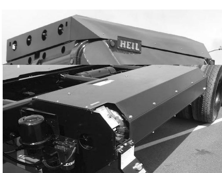
Figure 9. Compressed natural gas vehicle storage tank configurations: behind the cab, on the roof, or within the chassis
