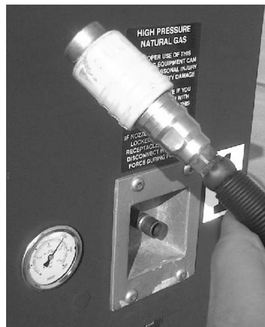
Figure 5. P36 CT1000 compressed natural gas push-pull actuating nozzle
